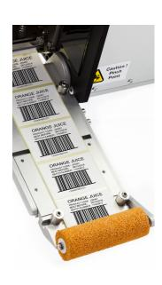
Specifically designed for group packaging labeling, meeting high volume production lines needs. APL 3500 F can print & apply up to 180 labels per minute.
